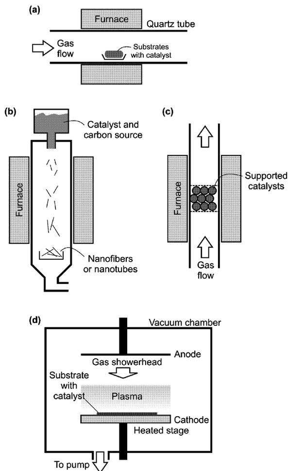
**Figure 6.** Types of chambers used for catalytic CVD of nanofibers and nanotubes. The most commonly used is the horizontal furnace (a). For mass production, the vertical furnace (b) has been employed. (c) The fluidized bed reactor and (d) a basic plasma enhanced CVD system based around a vacuum chamber.
