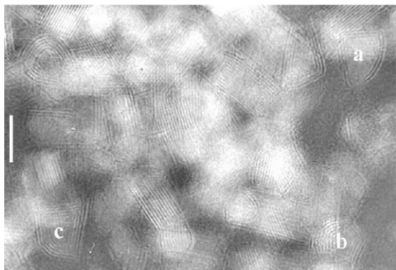
Fig. 1. Transmission electron microscopy image of \text{MoS}_2 nanoparticles generated using the arc in water. The particles labelled as a, b and c represent triangular, hexagonal and pentagonal projected shapes. The scale bar corresponds to 10 nm.
